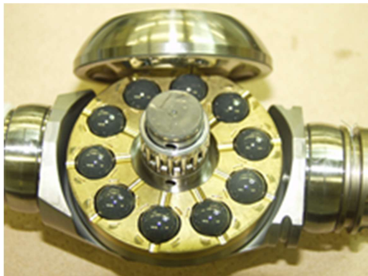
Figure 3-2. Photo of thrust ball bearing in power roller. Ceramic balls are applied.
