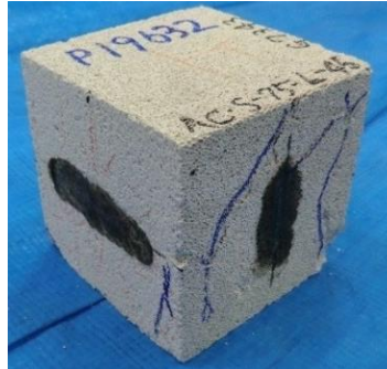
(b) 破壊性状① (A37-C-□75-M-0-D)
