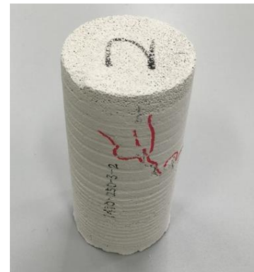
(f) 破壊性状① (A37-C-φ64-L-0-G-7)
