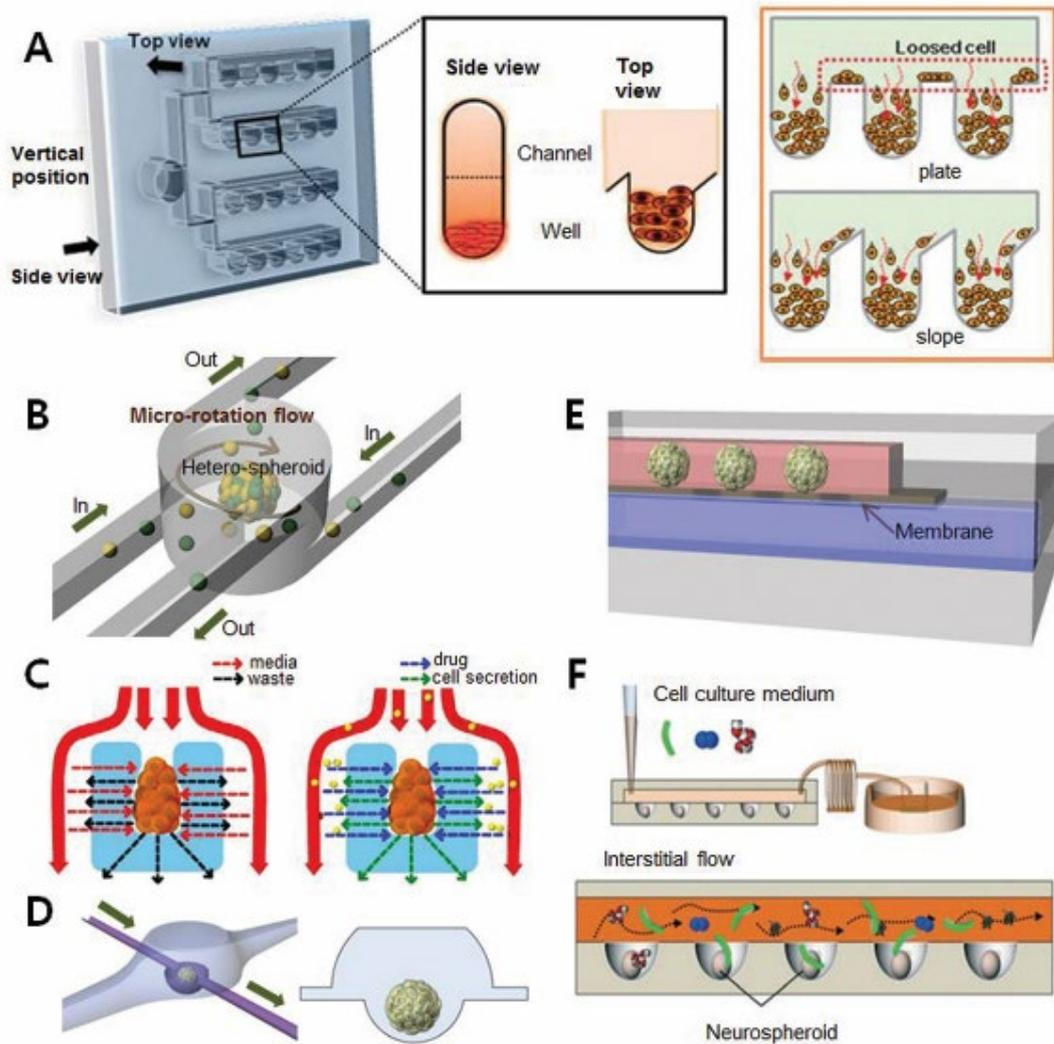
**Fig. 9. Schematic representation of different microfluidic systems.** A, F) Microfluidic chips with concave microwells, similar to the microwell arrays. B) Schematic representation of spheroid formation in a microfluidic device. C) A microfluidic device based on hydrodynamic trapping of cells in U-shaped geometries. D) A multilayer microfluidic device for culturing embryonic bodies. E) A microfluidic device based on semi-porous polycarbonate membrane<sup>25</sup>.
