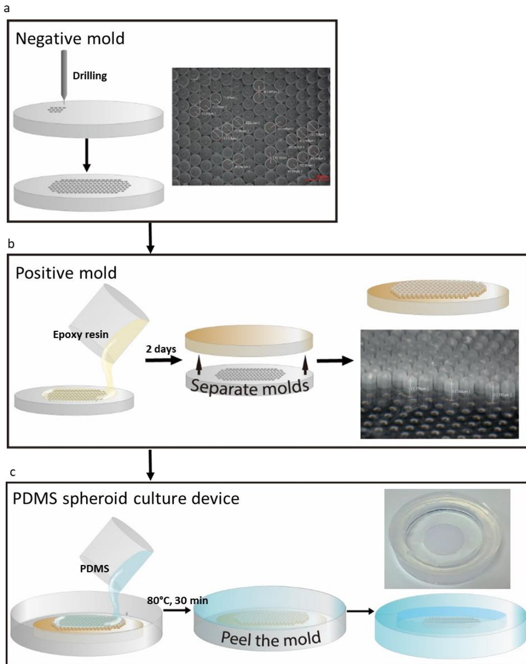
**Fig. 11. Fabrication of PDMS spheroid plate.** **a:** Fabrication of a negative mould by drilling wells in polystyrene circle and the photo of the resulted mould. **b:** fabrication of a positive mould by pouring epoxy resin solution onto the negative mould and the photo of the resulted mould. **c:** fabrication of PDMS-chip by pouring PDMS solution on positive mould and the photo of the final chip.
