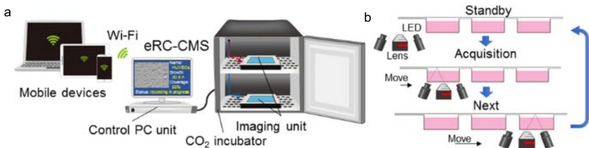
**Fig. 12. Flatbed *epi*-relief contrast cellular monitoring system (eRC-CMS).** **a:** the configuration of eRC-CMS, from right to left: the incubator for cell culturing equipped with objective lens and LEDs for *epi* relief-contrast imaging; the controlling PC with software that allows continuous monitoring of cells cultured in the incubator and sending collected data to another device by the network. **b:** the scheme of image acquisition.
