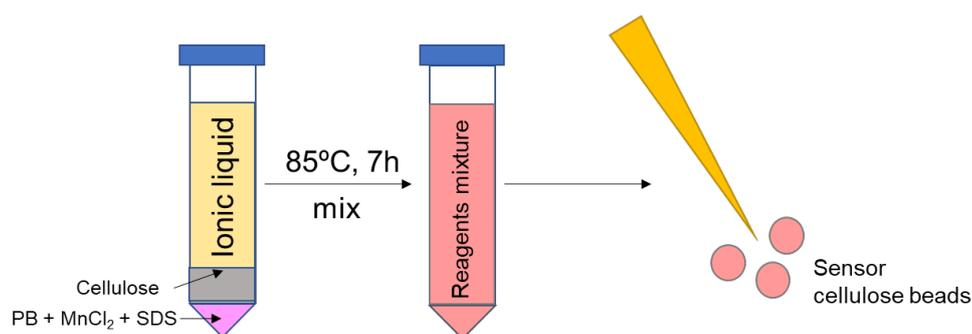
**Fig. 26.** Schematic representation of the fabrication of cellulose-ionic liquid hydrogel beads with immobilised reaction components for the determination of ROS.
