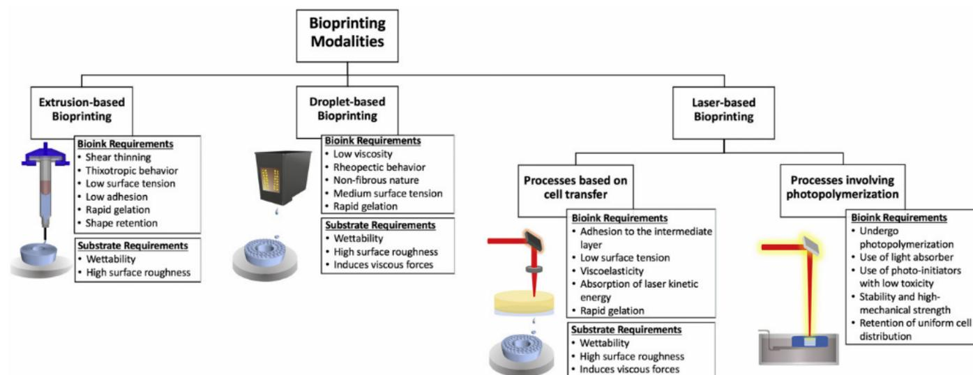
**Fig. 10.** Different types of bioprinters and requirements for utilised bioink<sup>30</sup>.
