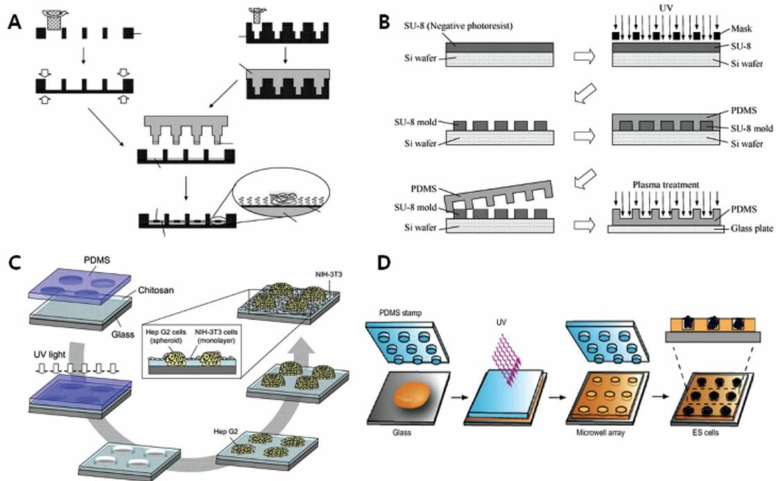
**Fig. 8. Several methods of microwell array fabrication.** A) PMMA replica is fabricated by the milling process. B) SU-8 replica is fabricated by photolithography. C, D) PDMS replica is fabricated by micromolding<sup>25</sup>.
