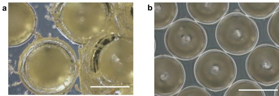
**Fig. 16. The examples of acrylic moulds of the same design made with the different speed parameters of a drill. a) x-y speed – 20%, z speed – 80%, rotation speed – 60%. b) x-y speed – 30%, z speed – 100%, rotation speed – 100%. Scale bar 500  $\mu$ m.**
