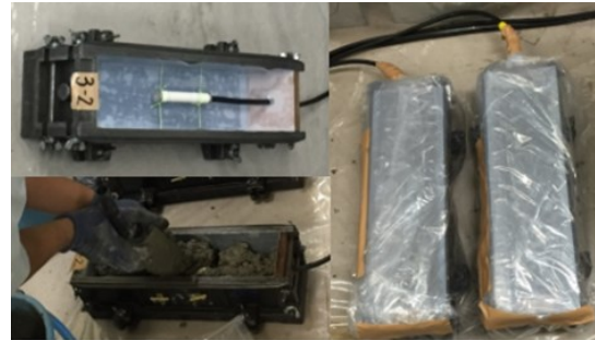
Fig.4.12(b) Autogenous shrinkage at 40°C curing temperature
