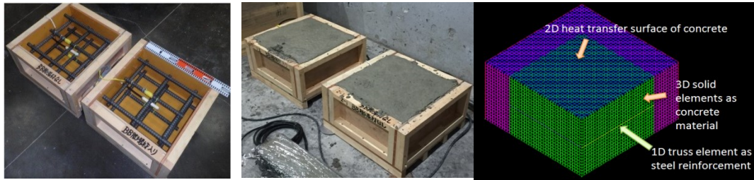
Fig.4.28(e) Small RC slab specimens and FEM model regarding Kosano RC slab concrete
