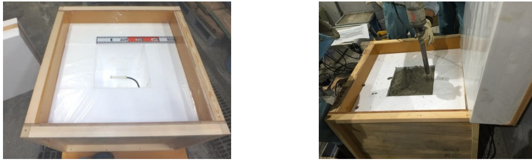
Fig.4.27(g) Kosano RC slab concrete specimen measuring autogenous shrinkage and concrete temperature rise due to hydration heat under semi-adiabatic condition
