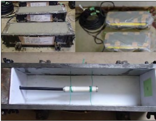
Fig. 4.35(c) Autogenous shrinkage specimens
