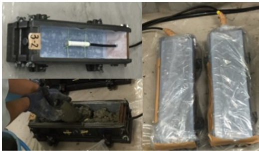
Fig.4.9(a) Autogenous shrinkage specimens with embedded type strain gauge
