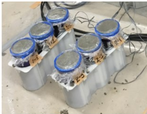
Fig.4.13(a) Expansion strain specimens in thin walled tinplated cylindrical steel molds
