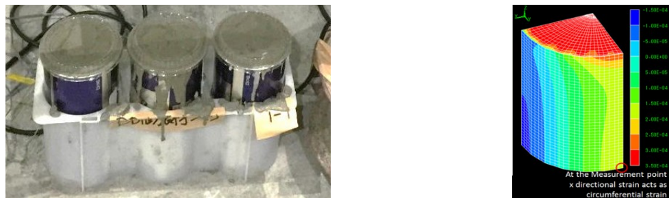
Fig.4.28(b) JCI-S-009-2012 cylindrical restrained expansion strain specimen and FEM model for Kosano RC slab concrete
