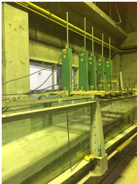
Fig. 4.16 Wave gauges stationed along the flat bed profile for wave height measurements during experiments
