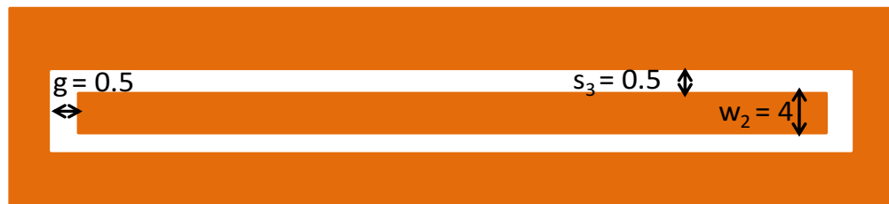
Fig. 3.20. Geometry of the simple CPW.
