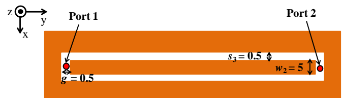
Fig. 7. Simple coplanar waveguide.
