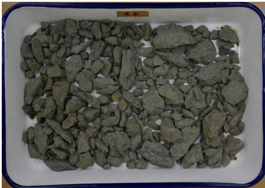
Figure 21. The mudstone specimen for accelerated slaking test (NEXCO-110-2012)
