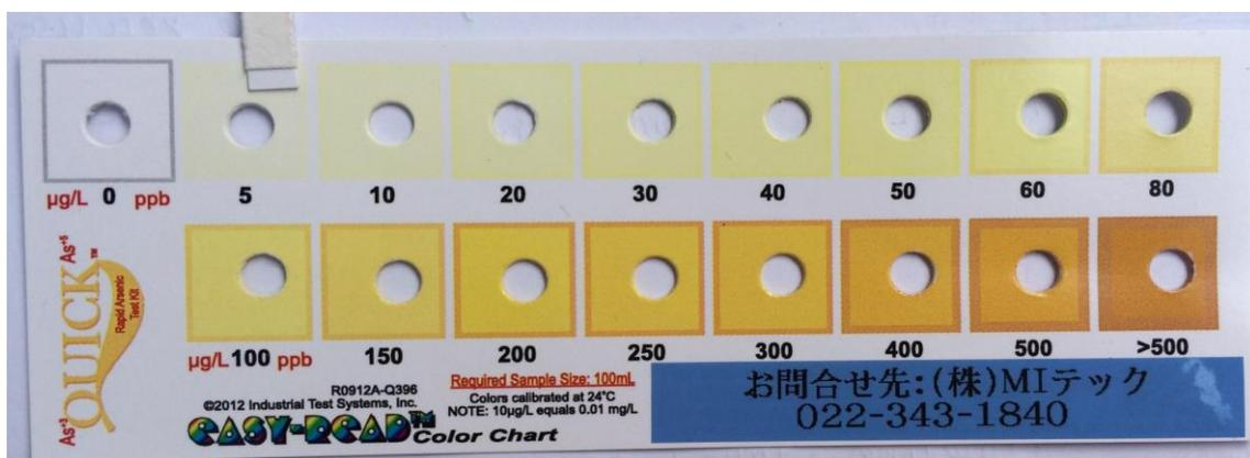
Fig. 2-3 Picture of the color of the test paper with standard color chart of the MITech arsenic test kit.
