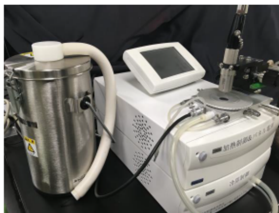
Fig. 3.3 Heating-cooling stage and Raman spectrometer
