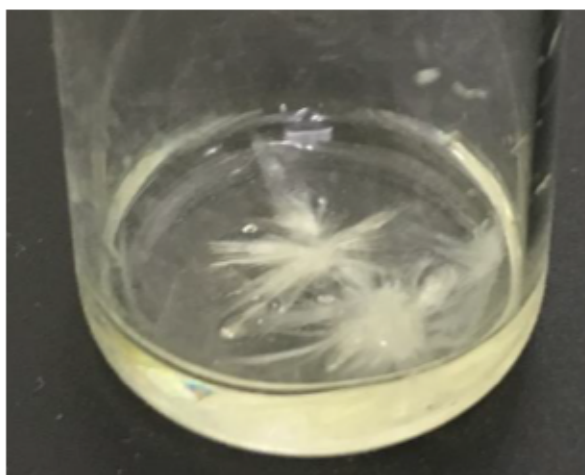
Fig.7.3 An ADN/MEAN/AA=60/20/20 (mass ratio) mixture at approximately 10 °C.
