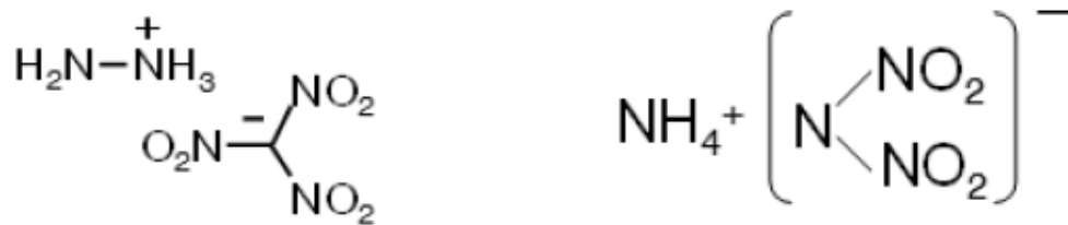
Fig.2.3 Molecular structure of HNF and ADN.
