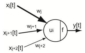
Fig. 1. Mathematical model of artificial neuron. f is the activation function of the neuron device. A three-input artificial neuron is shown.
