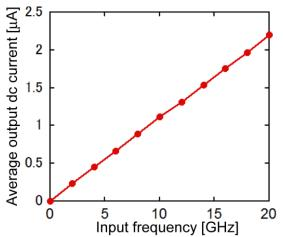
Fig. 6. Dependence of simulated average output current from frequency-tocurrent converter on the SFQ input frequency.
