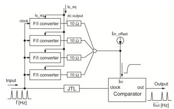
Fig. 7. Block diagram of test circuit of superconductive pseudo sigmoid function generator. The F/I converter corresponds to the frequency-to-current converter. Four frequency-to-current converters placed in parallel were used to supply a large dc current to the comparator.
