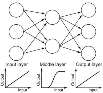
Fig. 2. Structure of artificial neural network, the perceptron. Each circle corresponds to an artificial neuron device. In the middle layer, devices having nonlinear input–output characteristics are required.
