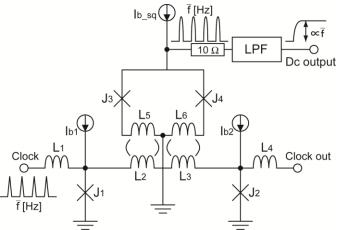
Fig. 5. Equivalent circuit of frequency-to-current comparator based on SFQ stochastic logic. An input SFQ pulse train is converted to dc current by the SQUID voltage generator and the low-pass filter (LPF).  $J_1 = J_2 = 216 \mu A$ ,  $J_3 = J_4 = 300 \mu A$ ,  $L_2 = L_3 = 12.5 \text{ pH}$ ,  $L_5 = L_6 = 14.0 \text{ pH}$ ,  $I_{b1} = I_{b2} = 150 \mu A$ .
