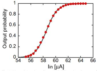
Fig. 4. Measured dependence of output probability on input dc current of SFQ comparator. The dots represent the measurement results. The solid line represents the fitting sigmoid function.
