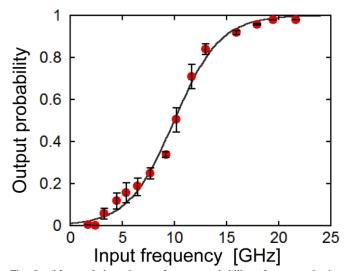
Fig. 8. Measured dependence of output probability of superconductive pseudo sigmoid function generator on input frequency. The dots represent the measurement results. The solid line represents the fitting sigmoid function.
