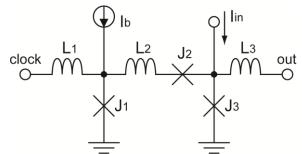
Fig. 3. Equivalent circuit of SFQ comparator.  $L_1$  =2.5 pH,  $L_2$  = 5.0 pH,  $J_1$  =  $J_2$  =  $J_3$  = 216  $\mu$ A,  $I_b$  = 150  $\mu$ A.
