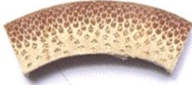
Fig. 1.3.1 Gradient distribution of longitudinal fibrous structure of bamboo [32]
