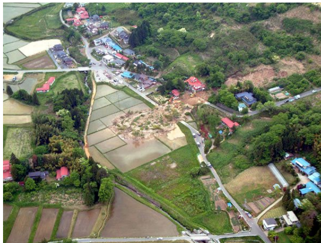
Figure 1.2 Landslide due to liquefaction in Tsukidate, 2003 (Photo by Prof. Kazuo Konagai)
