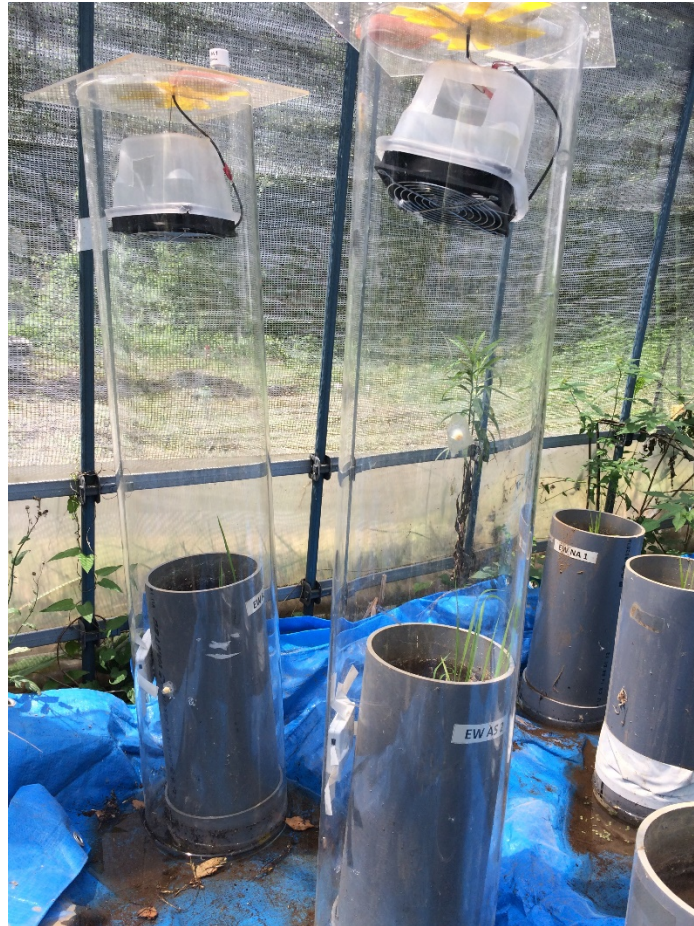
Photo 10: Gas sampling by closed chamber method
