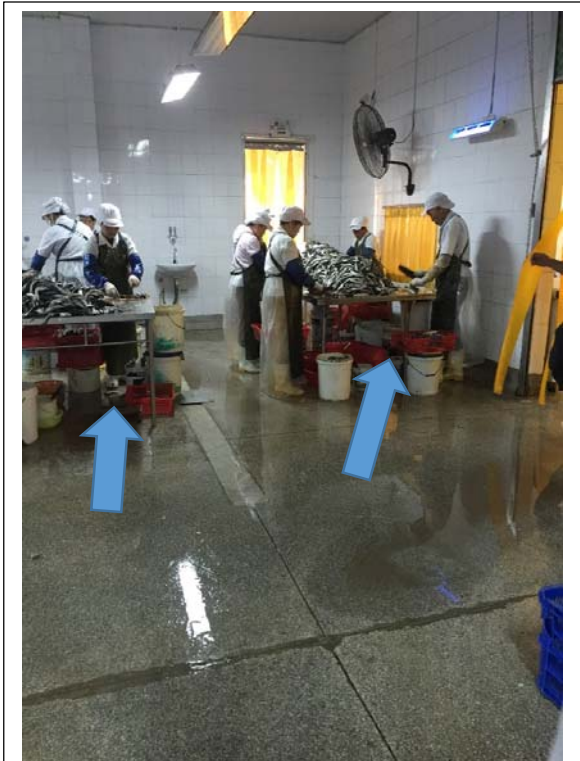
Figure 5.8 a. Solid waste drained into wastewater due to manually headed and gutted step
