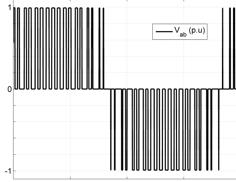
Figure 3-4: Output line-to-line voltage of a three phase inverter.
