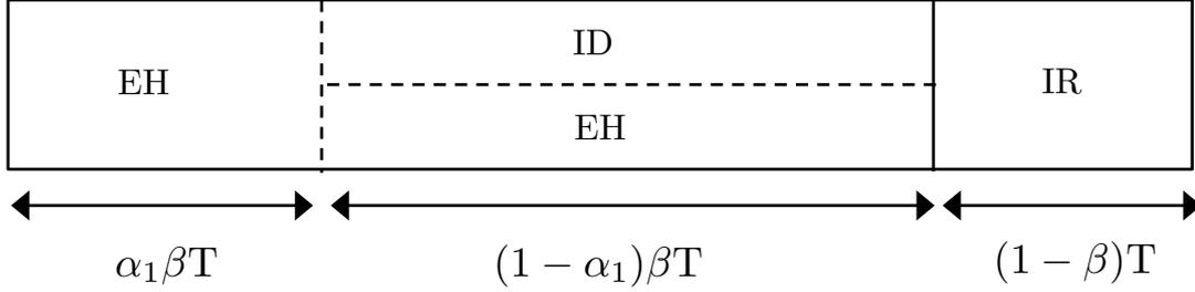
Figure 4.3: A block structure of the ATS-APS protocol.
