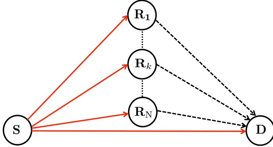
Figure 2.3: Cooperative network with multiple relay nodes
