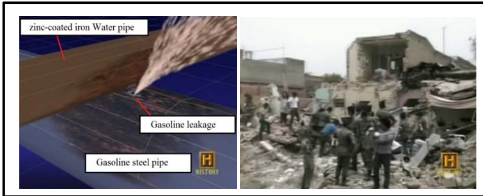
Fig. 2- Explosion in Guadalajara caused by corrosion of gasoline pipeline [11].
