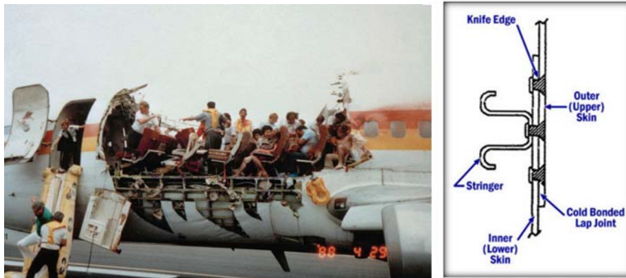
(a) Failure of Boeing 737 at the upper fuselage (b) Lab joints upper fuselage
