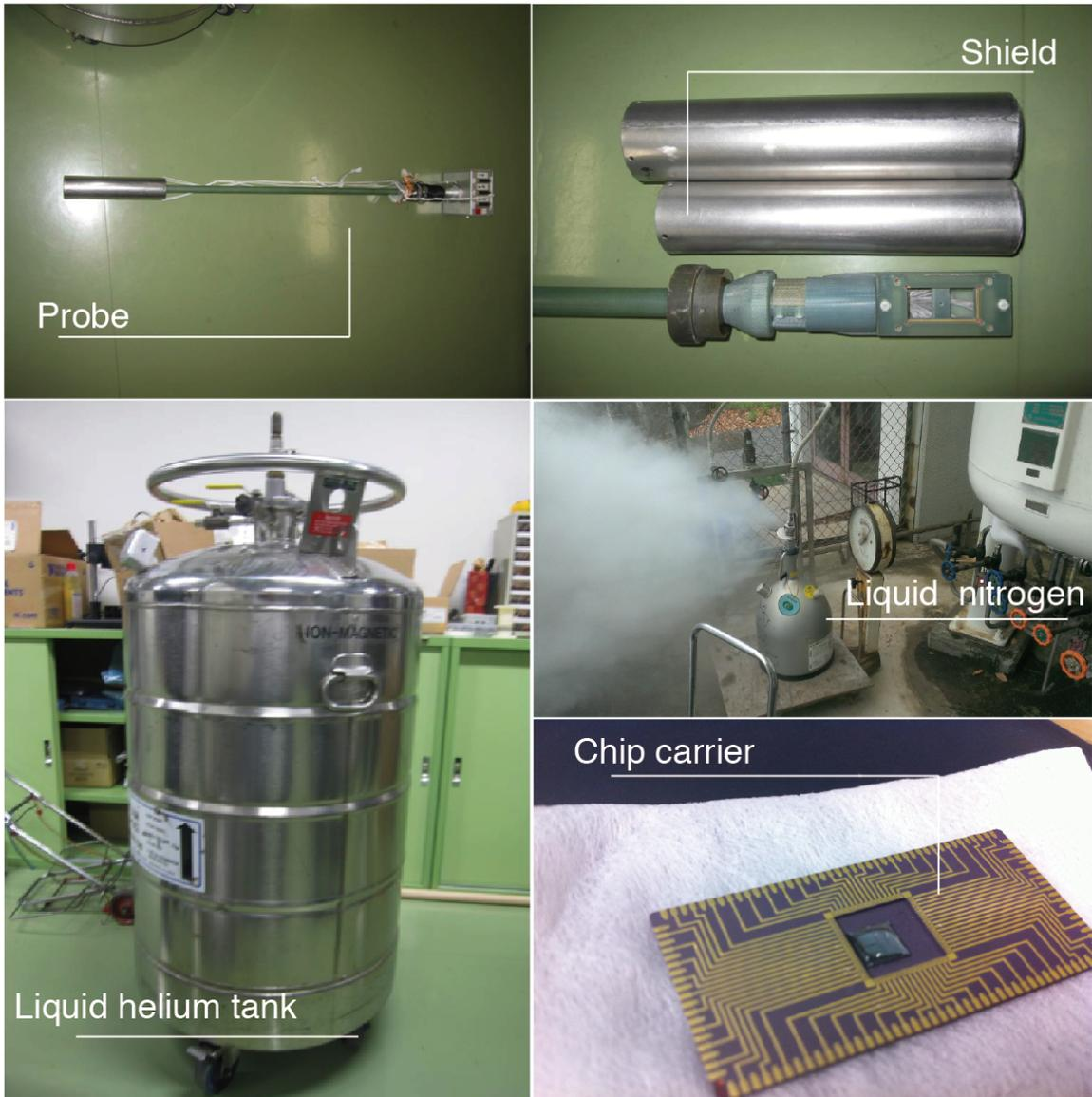
Figure 3-10: Details of measurement system.
