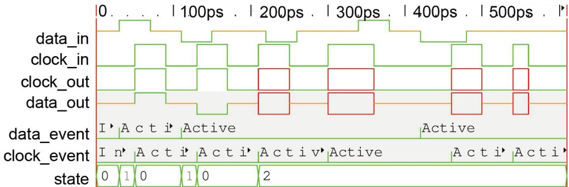
Figure 4-21: Example of simulated waveforms of several cases with different timing variations. The first two error outputs are generated because of the early arrival of clock before data, whereas the third one is reported by the late clock arrival time and the last error indicates there is no data signal exits when clock arrives.
