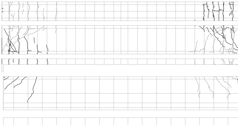
Fig (A.8) Cracks pattern of SP-S3
