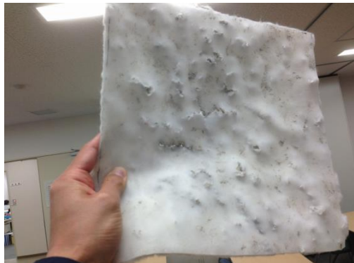
Figure 3.16 Damaged EVA sheet in the bottom parts of the second lining
