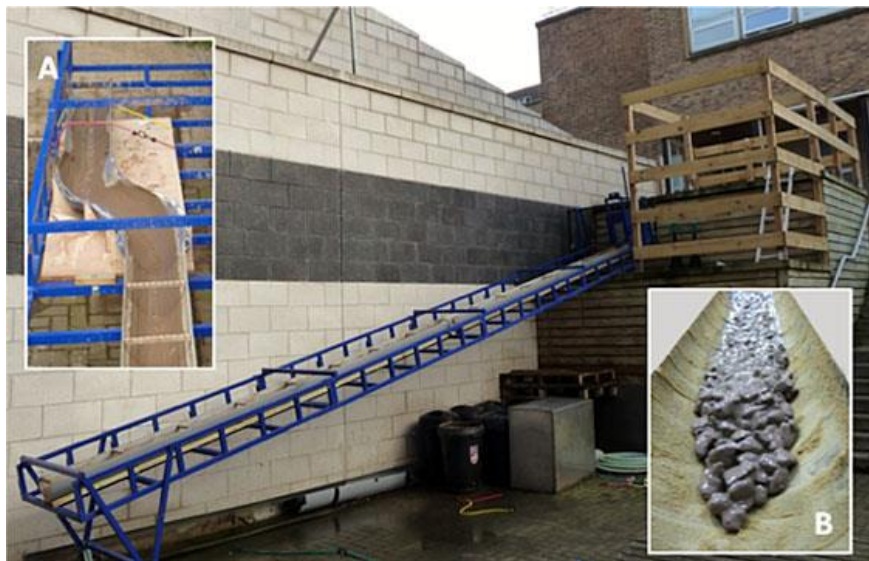
Fig 2.9 A curved flume for debris flow analysis (Source: Durham University)
