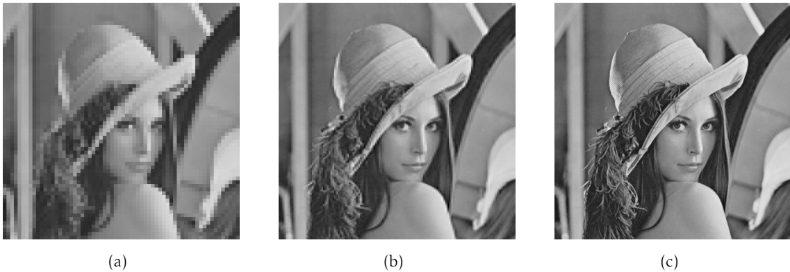
Figure 2.4: Lena images with multiresolution. (a) From 1 DCT coefficients, PSNR=23.21 dB. (b) From 5 DCT coefficients, PSNR=27.82 dB. (c) Full resolution.
