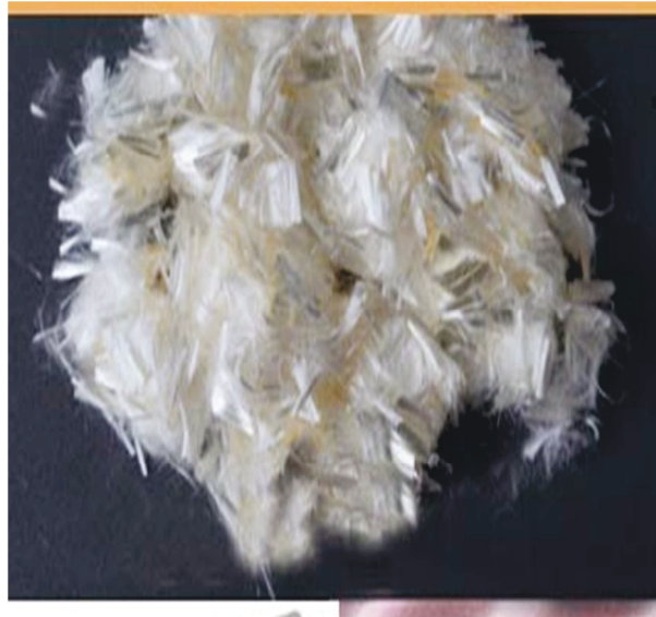
Fig C.9 High tenacity and high modulus PVA fiber (Type-C) 92) .
