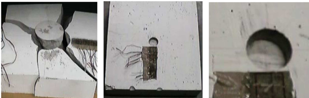
Fig. 1.5 Failure modes of a) Mortar slab b) PVA-ECC slab and c) Close up view near indent 6)
