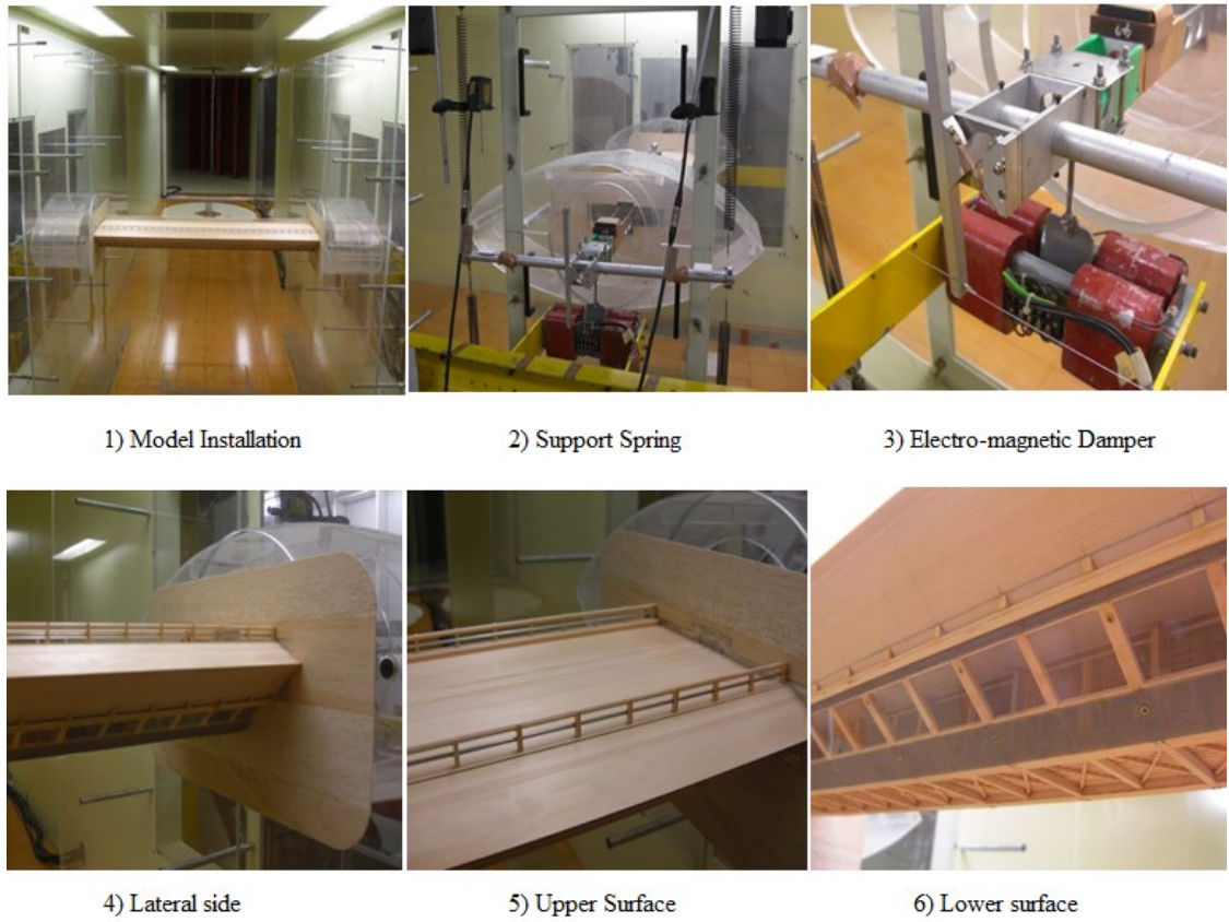
Figure 4.8. String supported model of the Shin-minato Bridge in WTT [7]
