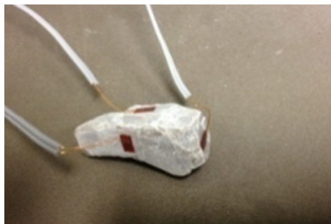
Fig. 3.9 Measurement of CTE of coarse aggregate.
