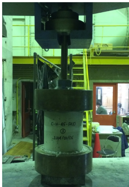
Fig. 3.10 Direct tensile strength test of concrete.
