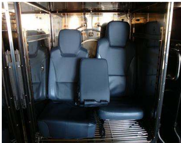
Fig.4-1 Measuring VOCs emitted from inner components using chamber.
