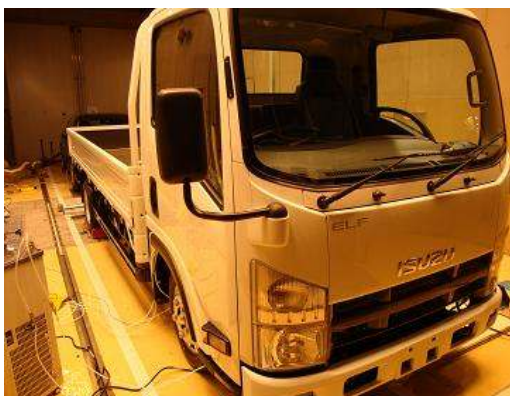
Fig.3-2 Evaluation of temperature under JASO Z125
