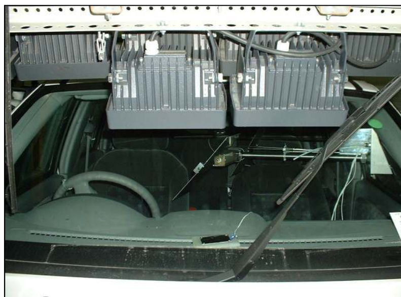
Fig.2-4 Heating system of FAT AK26
