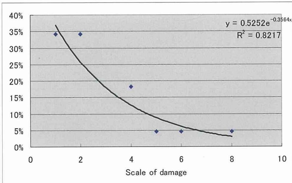
Figure 4. 9 Distribution of the scale of damage for Strong winds with regression curve
