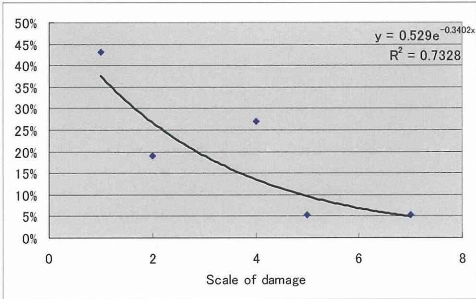
Figure 4. 10 Distribution of the scale of damage for Flooding with regression curve
