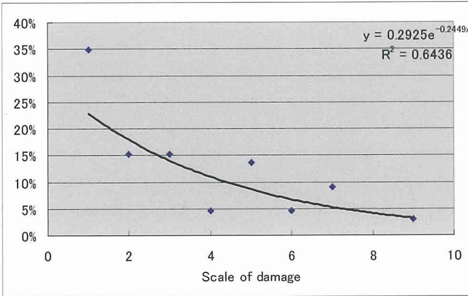
Figure 4. 8 Distribution of the scale of damage for Fire/Explosion with regression curve
