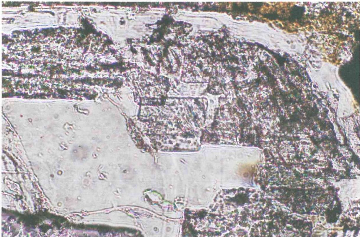
Fig. 4-2-2; Plagioclase phenocryst includes glass zone and clear rim. Result for line analysis along the blue line shows the graph. Red line is the scale (1mm).
