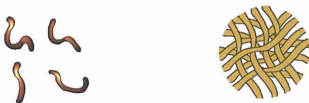
Figure 1.2: Schematic diagram of non-entangled (concentration < c^* ), and entangled (concentration > c^* ) wormlike micelles.
