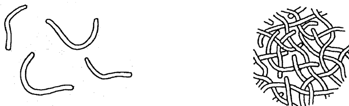
Figure 1-9: Schematic diagram of unentangled ( concentration < c^* ) and entangled ( concentration > c^* ) worm-like micelles.
