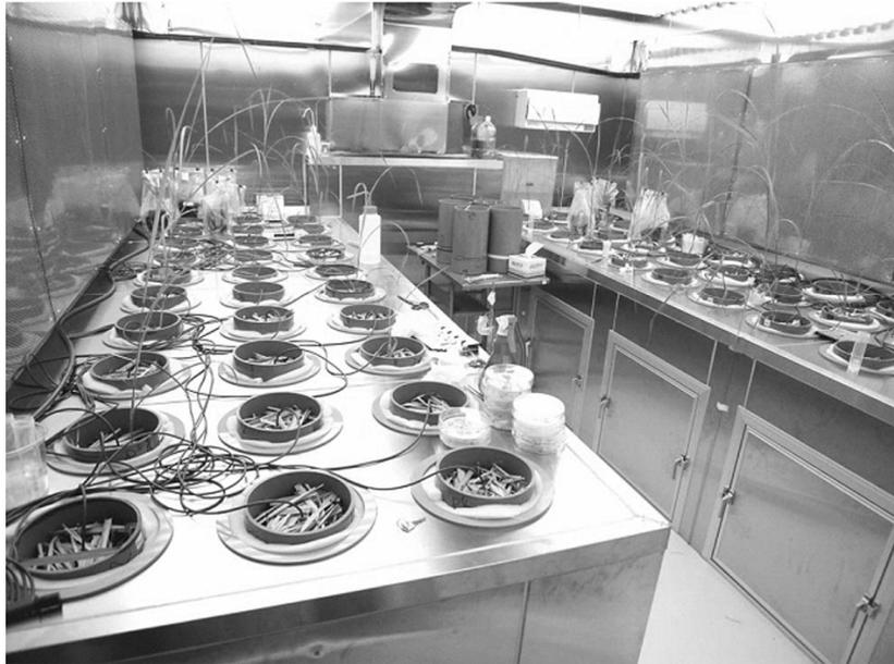
Fig. 1 The Earthtron facility. Two cabinets are fixed to opposite sides of the chamber. The cabinets can be assigned with experimental pots (the experiment shown in this photograph is not the present study)
