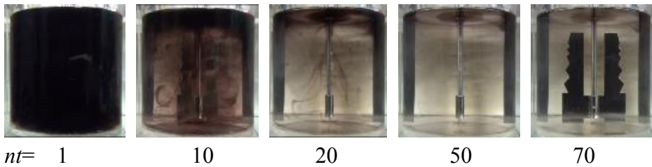
Fig. 5.145 Mixing patterns obtained with a Supermix MR203 in a baffled flat vessel ( Re=80 ; \rho=1308\text{kg/m}^3 \mu=0.115\text{ Pa}\cdot\text{s} n=49\text{rpm} )
