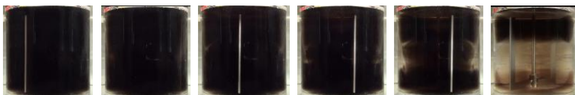
Fig. 5.153 Mixing patterns obtained with an Anchor ( Re=15; \rho=1363\text{kg/m}^3 \mu=0.960 \text{ Pa}\cdot\text{s} n=23\text{rpm} )
