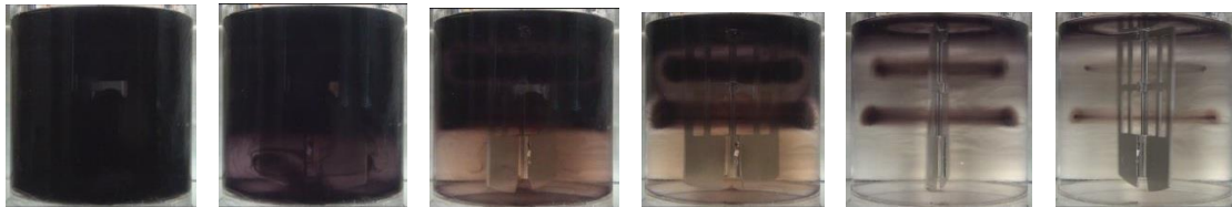
Fig. 5.8 Mixing patterns obtained with a Maxblend in an unbaffled flat vessel ( Re=25 ; \rho=1347\text{kg/m}^3 \mu=0.48\text{ Pa}\cdot\text{s} n=38\text{rpm} )
