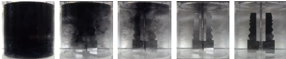
Fig. 5.137 Mixing patterns obtained with a Supermix MR203 in an unbaffled flat vessel ( Re=600 : \rho=1235\text{kg/m}^3 \mu=0.020\text{ Pa}\cdot\text{s} n=54\text{rpm} )
