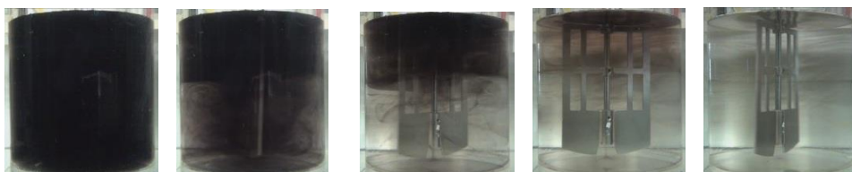
Fig. 5.10 Mixing patterns obtained with a Maxblend in an unbaffled flat vessel ( Re=100 ; \rho=1308\text{kg/m}^3 \mu=0.115\text{ Pa}\cdot\text{s} n=37\text{rpm} )
