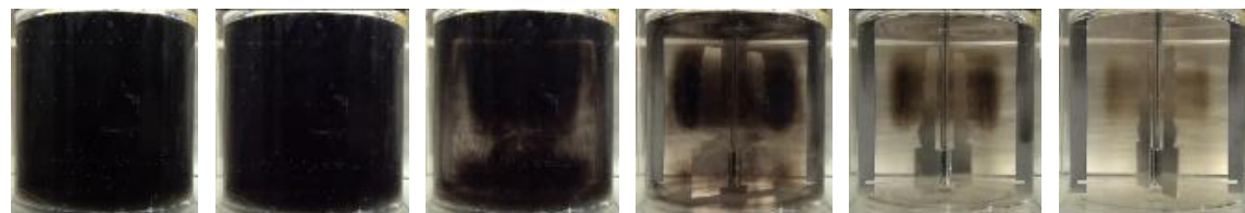
Fig. 5.139 Mixing patterns obtained with a Supermix MR203 in an unbaffled flat vessel ( Re=3000 : \rho=1175\text{kg/m}^3 \mu=0.008\text{ Pa}\cdot\text{s} n=113\text{rpm} )
