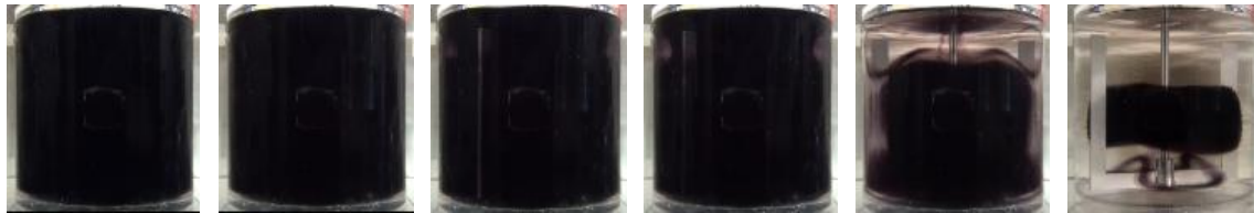
Fig. 5.151 Mixing patterns obtained with an Anchor ( Re=6; \rho=1368\text{kg/m}^3 \mu=2.5 \text{ Pa}\cdot\text{s} n=24\text{rpm} )
