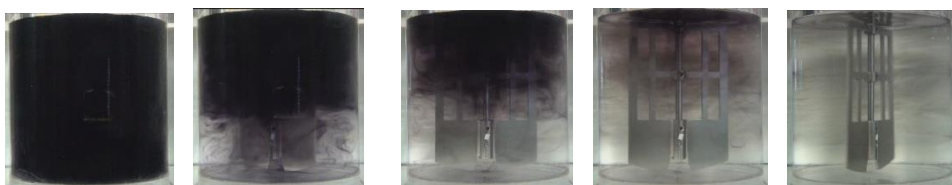
Fig. 5.11 Mixing patterns obtained with a Maxblend in an unbaffled flat vessel ( Re=240 ; \rho=1280\text{kg/m}^3 \mu=0.054\text{ Pa}\cdot\text{s} n=43\text{rpm} )
