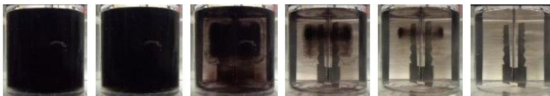
Fig. 5.140 Mixing patterns obtained with a Supermix MR203 in a baffled flat vessel ( Re=6 : \rho=1370\text{kg/m}^3 \mu=1.600\text{ Pa}\cdot\text{s} n=39\text{rpm} )
