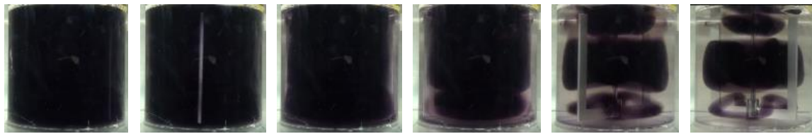
Fig. 5.151 Mixing patterns obtained with an Anchor ( Re=6; \rho=1368\text{kg/m}^3 \mu=2.5 \text{ Pa}\cdot\text{s} n=24\text{rpm} )
