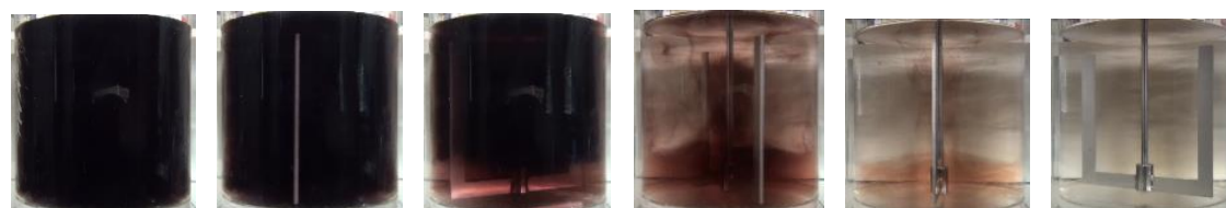
Fig. 5.155 Mixing patterns obtained with an Anchor ( Re=40; \rho=1336\text{kg/m}^3 \mu=0.300 \text{ Pa}\cdot\text{s} n=20\text{rpm} )
