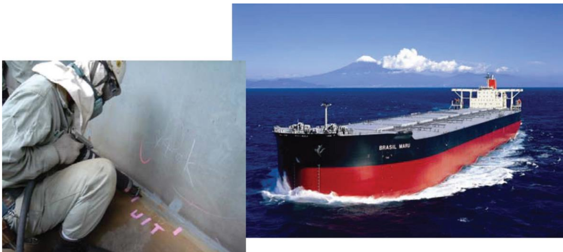
Figure 1.2 UIT treatment in 320,000 ton ore carrier "Brazil Maru" (Nose & Okawa [4]).
