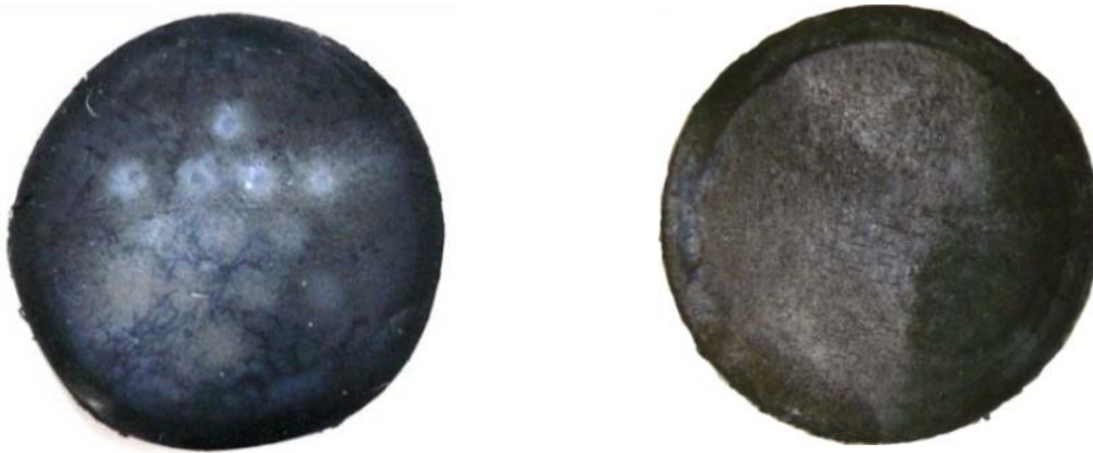
(a) Gap width of 0.1mm between films (b) Gap width of 1.0mm between films
