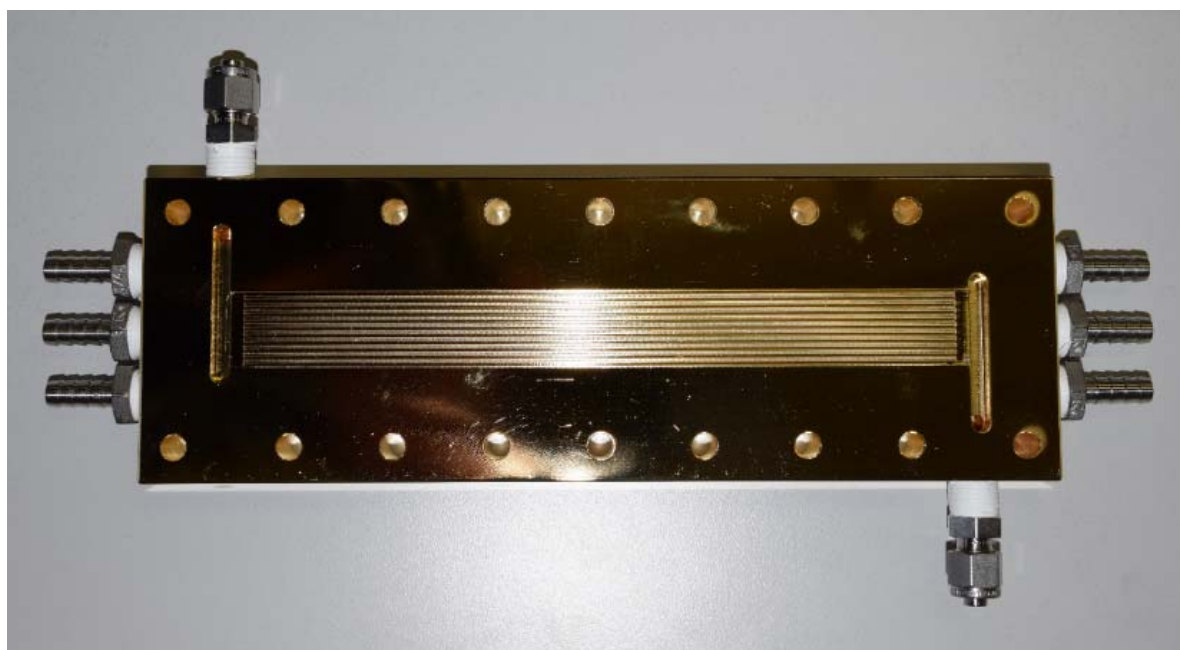
Fig. 4.7 Separator of PEFC (gold-plated brass)
