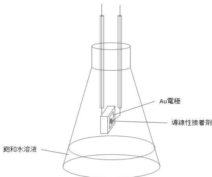
Fig. 9-1-5 The experimental setup to keep the relative humidity, 笠井, 修論 (2012) p.24
