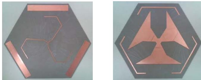
Figure 3. 22 Fabricated sample of the notched array antenna with parasitic elements.
