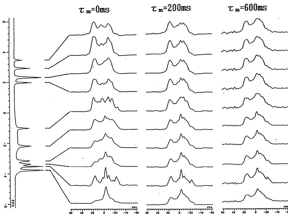
Figure 5 Dependence of the cross sectional patterns on the mixing time  $\tau_m$  of 0, 200, 600 ms in the SC-2D NMR spectrum of EBBA.
