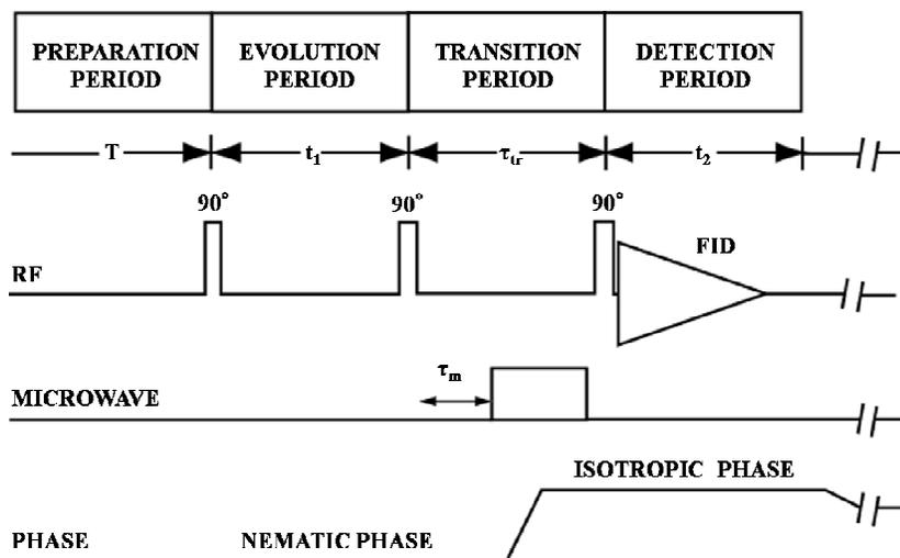
*Figure 2 Pulse sequence for the state-correlated 2D NMR (SC-2D NMR) experiments. A mixing time  $\tau_m$  is inserted into the beginning of a transition period to examine the spin diffusion properties.*
