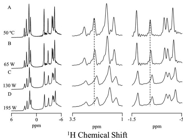
**Fig. 4**  $^1\text{H}$  NMR spectra (left) and expanded spectra (middle and right) of MBBA in the isotropic phase at (A) 50 °C and under CW microwave irradiation of (B) 65, (C) 130 and (D) 196 W for 10 min while regulating the instrument temperature at 50 °C.
