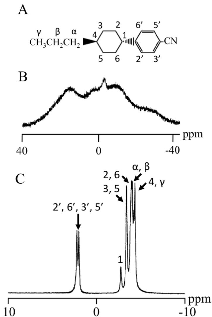
Fig. 2. (A) Molecular structure of PCH3.  $^1\text{H}$  NMR spectra of PCH3 measured at (B) 40 °C in the liquid crystalline phase and at (C) 50 °C in the isotropic phase. High resolution  $^1\text{H}$  NMR signals were assigned to individual protons as indicated [21].
