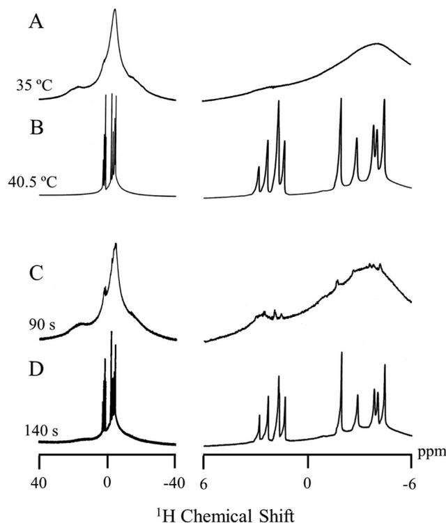
Fig. 2  $^1\text{H}$  NMR spectra (left) and expanded spectra (right) of MBBA at (A) 35 and (B) 40.5 °C and setting the temperature at 20 °C under 130 W CW microwave irradiation for (C) 90 and (D) 140 s.
