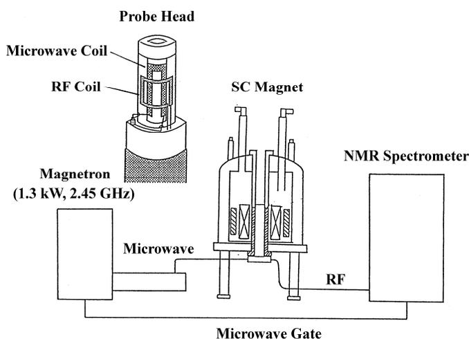
*Figure 1 Block diagram of the microwave heating NMR spectrometer equipped with a microwave transmitter. Microwave and radiowave coils in the probe head are also shown.*
