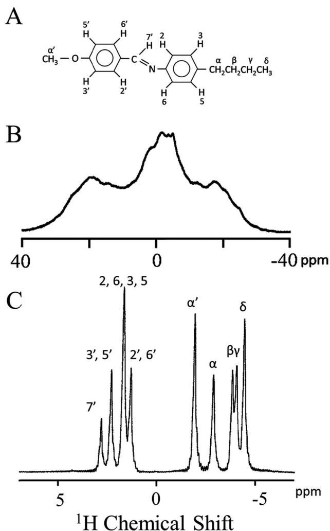
Fig. 1 (A) Molecular structure of *N*-(4-methoxybenzylidene)-4-butylaniline (MBBA).  $^1\text{H}$  NMR spectra of MBBA at (B) 35 °C in the liquid crystalline phase and (C) 45 °C in the isotropic phase, together with signal assignments of the individual protons.<sup>36</sup>
