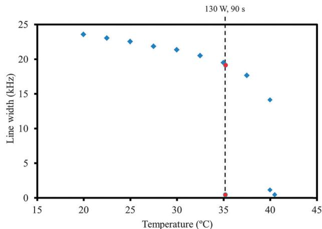
**Fig. 3** Plot of the line widths of  $^1\text{H}$  NMR spectra of MBBA at various temperatures as regulated by the instrument temperature control unit (blue square). The red square indicates the temperature (35 °C) of MBBA in the liquid crystalline state following microwave irradiation at 130 W for 90 s, in which a small amount of isotropic phase appeared within the liquid crystalline bulk.
