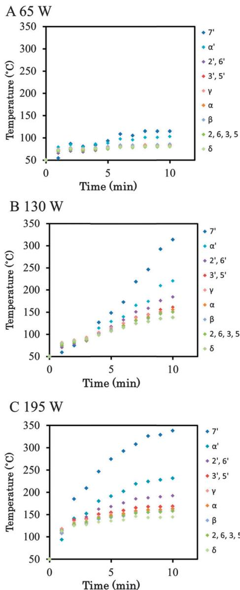
Fig. 6 Plots of temperatures against microwave irradiation time at microwave powers of (A) 65, (B) 130 and (C) 195 W. Temperatures were determined using the slopes obtained for the individual protons.
