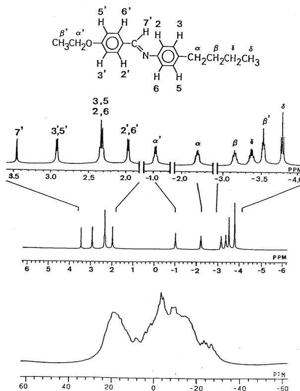
Figure 3  $^1\text{H}$  NMR spectra of EBBA in the isotropic phase at  $82^\circ\text{C}$  (top) and in the nematic phase at  $78^\circ\text{C}$  (bottom). The expansion of the top spectrum is shown above the spectrum of isotropic phase with signal assignments.
