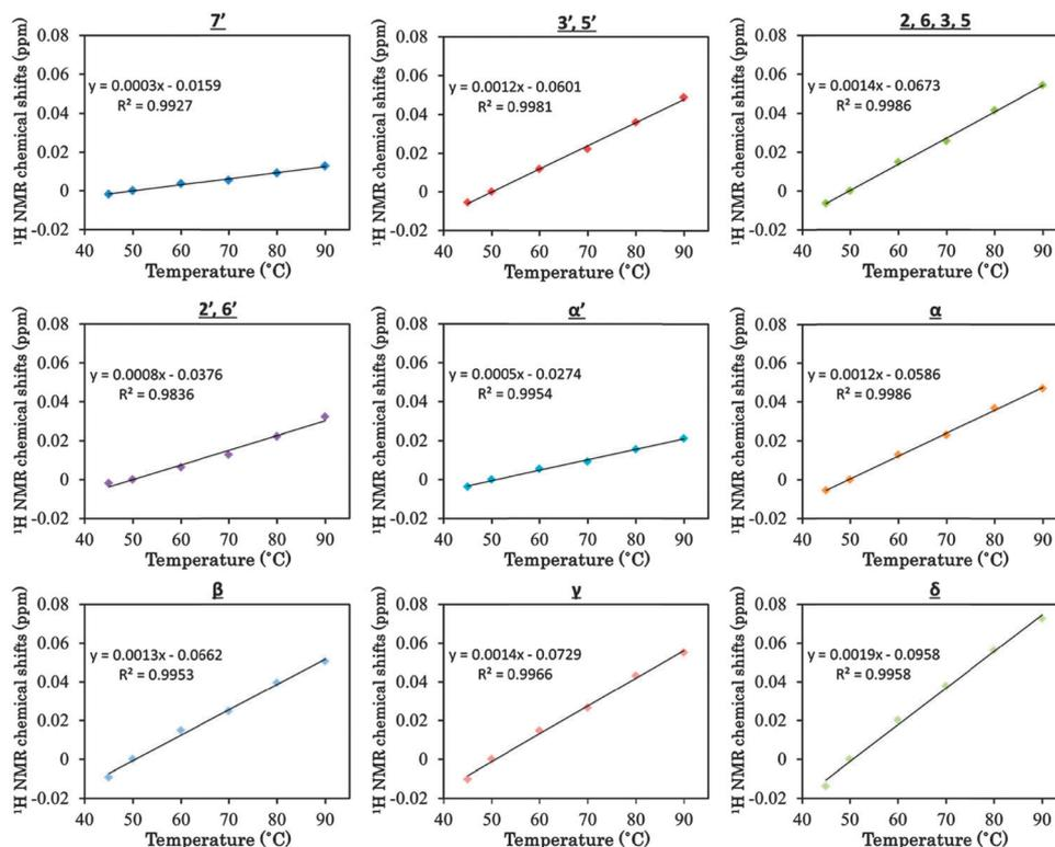
Fig. 5 Plots of <sup>1</sup>H chemical shift values of MBBA for individual protons against temperatures regulated by the instrument's temperature control system.
