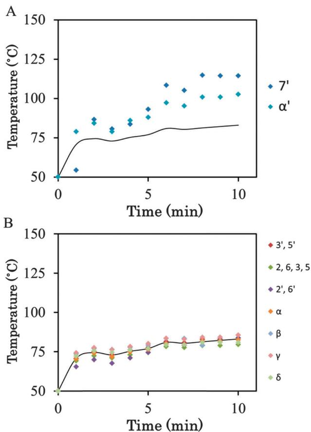
Fig. 7 Plots of temperatures against microwave irradiation times under microwave irradiation at 65 W for (A) the 7' and  $\alpha'$  protons (blue symbols) and (B) the remainder of the protons. The black line in both plots indicates the average temperature of the remainder of the protons.
