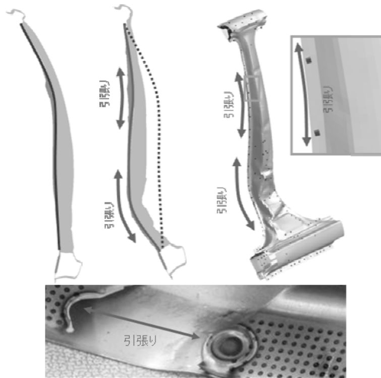
Fig. 6.15 The deformation mode of the center pillar part and example of spot-weld fracture
