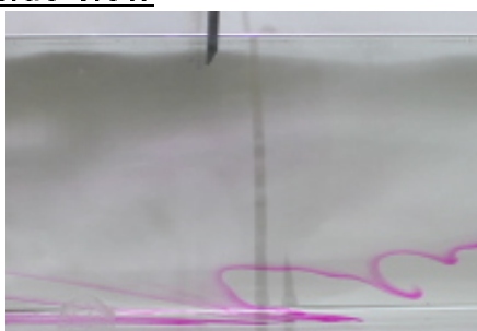
Fig. 4.4 Result of the injected tracer flow visualization, viscosity: 500 mPa·s, flow rate: 0.933 mm/s, tracer injection point: H/2, impeller: six-blade flat paddle impeller, rotational speed: 15 rpm
