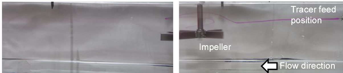
Fig. 4.9 Result of the injected tracer flow visualization, viscosity: 500 mPa·s, flow rate: 0.933 mm/s, tracer injection point: (3/4)H, impeller: six-blade flat paddle impeller, rotational speed: 35 rpm
