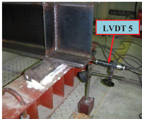
(c) Displacements measurement at the rear support
