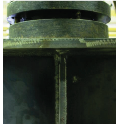
Buckling in Stiffener
