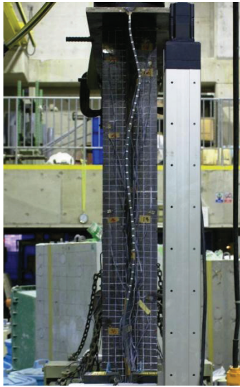
Figure 4.13: Failure mode of specimen S60U50
