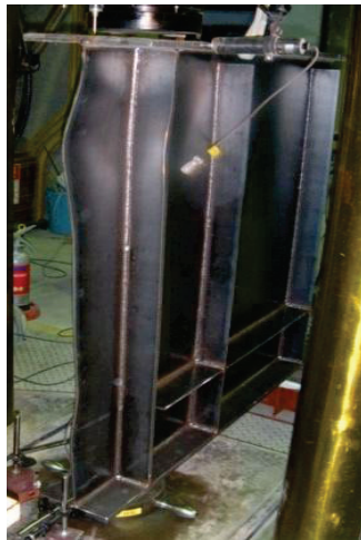
Figure 4.10: Failure mode of Healthy specimen
