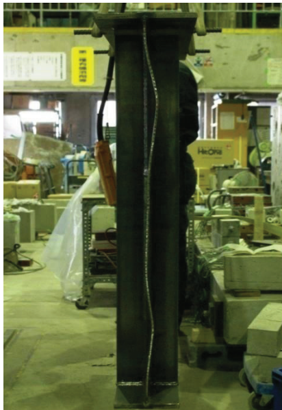
Figure 4.12: Failure mode of specimen S20N50
