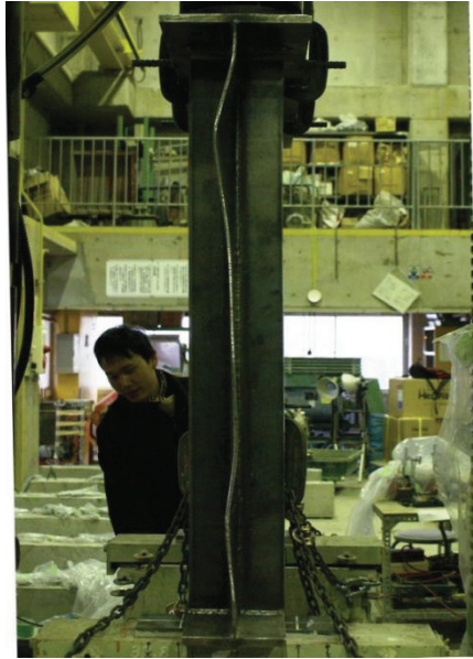
Figure 4.11: Failure mode of specimen S20U50
