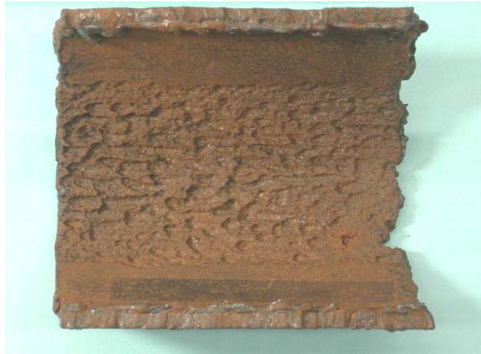
Fig. 1-10 Typical CO 2 corrosion of carbon steel
