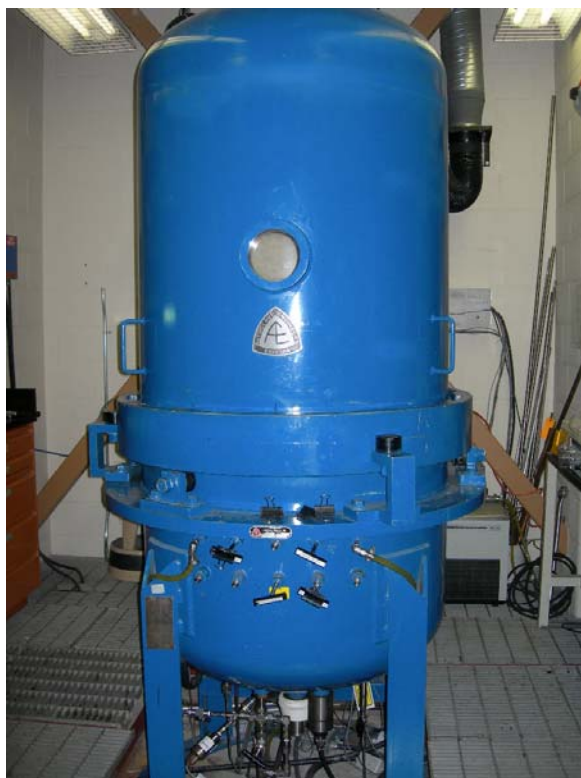
Fig. 4-1 H 2 S flow loop test apparatus at high temperature and high pressure
