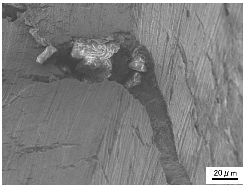
Fig. 5-8 Microcracks initiated pitting corrosion for 15Cr SS, 4.17 \times 10^{-7} \text{ sec}^{-1} , 180^\circ\text{C} , \text{CO}_2 3MPa, chloride ion 20,000ppm
