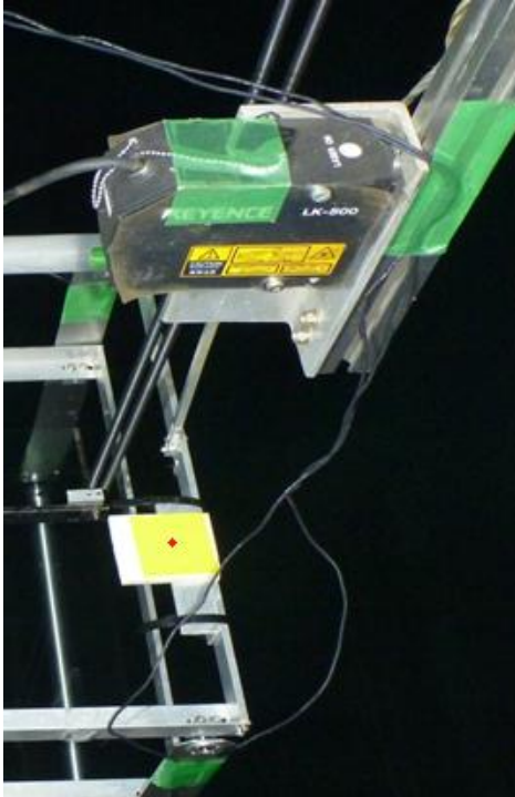
Figure 3.8: Laser displacement measurement device positioned over the cylinder.
