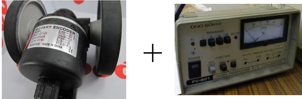
Figure 3.11: Rotatory encoder and frequency/voltage converter used to measure the towing carriage speed.
