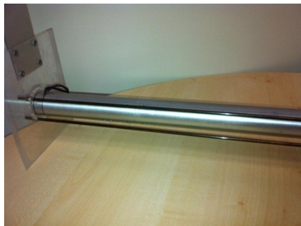
Figure 3.5: Cylinder and tripping wires connected to the endplate.
