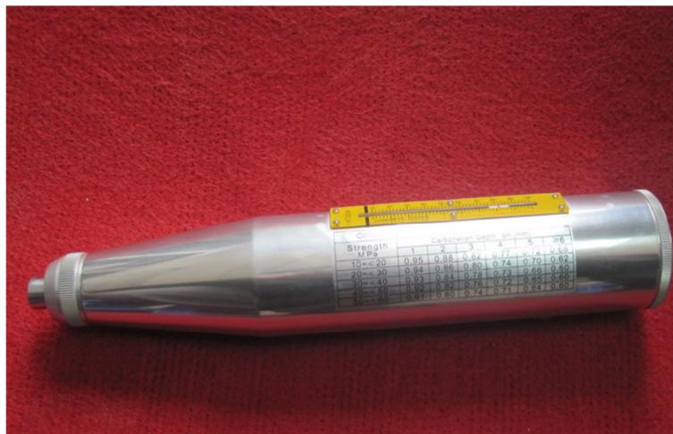
**Fig. A.1** Concrete test hammer [A.1]
