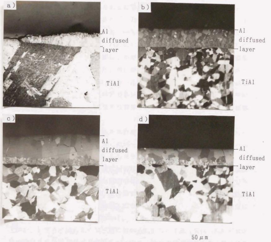
Fig.3.4 Cross-sectional micrographs of surface layer formed on TA and F-TA specimens by Al-diffusion coating.
