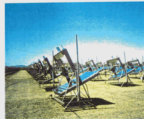
Photo.5.2 Accelerated outdoor exposure test (EMMAQUA)
