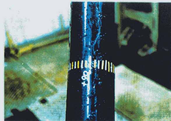
Photo.6.5 Water rivulets on upper surface of model C2
