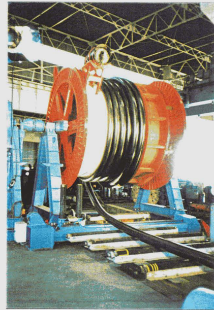
Photo.4.2 Unreeling test of a pre-coated parallel wire cable
