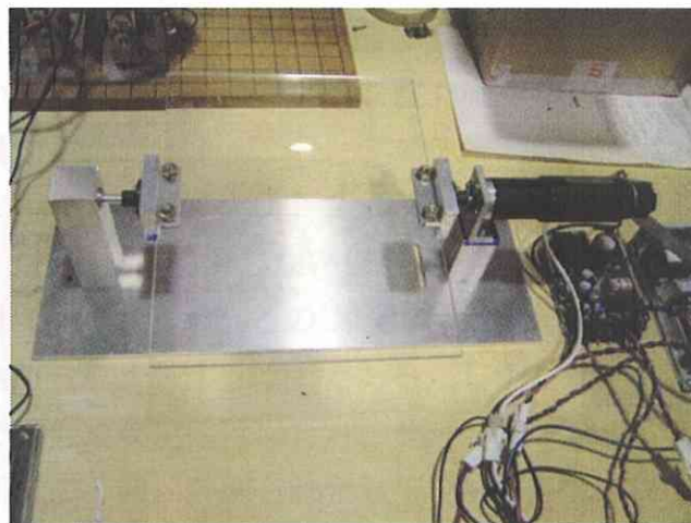
Fig. 3.6 Platform: This platform consists of three parts; one is motor, another is connection part with PC, and the other is plate that has low friction level. Therefore, the plate is covered with rubber.
