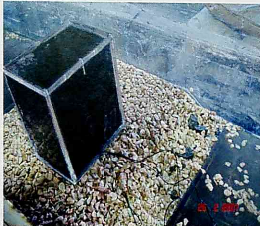
Fig. 3.5: View of the back of the rubble mound foundation.
