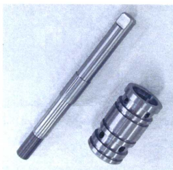
Photo 4-2 Piston with feedback slot (Left) and sleeve (Right)
