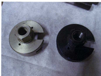
Photo 4-3 Coupling (Left; Aluminum, Right; Steel)
