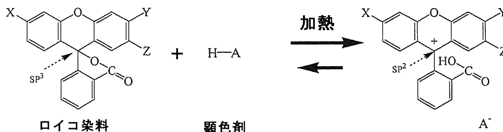
Figure 1-8 Color developing mechanism. (Conventional form)
